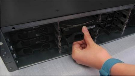
5. Attach the front panel and secure it with screws.
