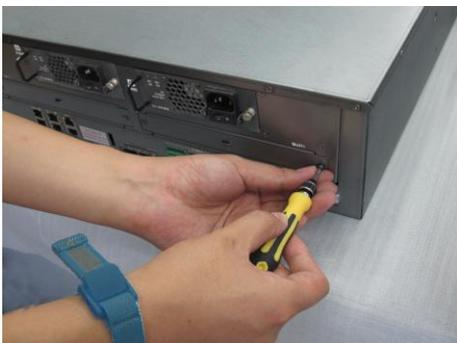
2. Insert the decoding card in place.
