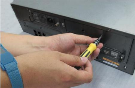
2. Insert the power module in place.
