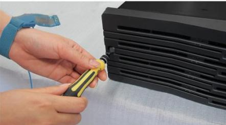
3. Align the hard disk with the slot and push in the disk gently.
